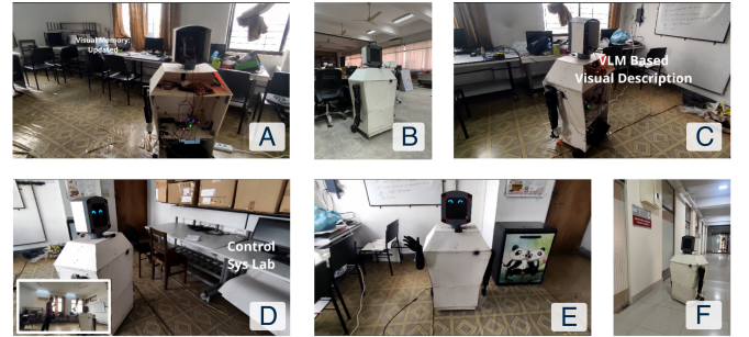
Fig. 6. Real-world implementation and experimental evaluation of the proposed architecture on a custom robotic platform: (A) vLM invocation for visual understanding; (B) autonomous navigation within an indoor laboratory environment; (C) visual memorization using agentic vLM calls for future spatial recollection; (D) chauffeuring the user to a requested destination; (E) spontaneous user greeting based on predicted mood and perceived direction of communication; and (F) navigation through a narrow corridor while describing the surroundings to maintain user engagement.
