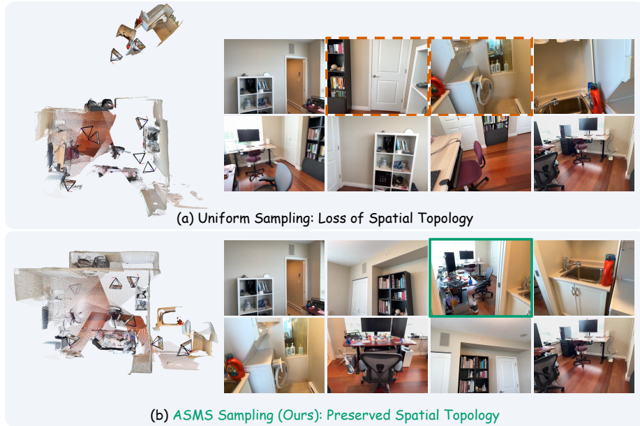
Fig. 4: Qualitative comparison between ASMS and uniform sampling under a sparse 8-frame setting. (a) Uniform sampling misses key spatial transitions (dashed orange boxes), resulting in topological disconnection and a fragmented point cloud. (b) Our ASMS adaptively captures crucial bridge frames (solid green box) to preserve the global spatial topology, yielding a coherent scene structure.
