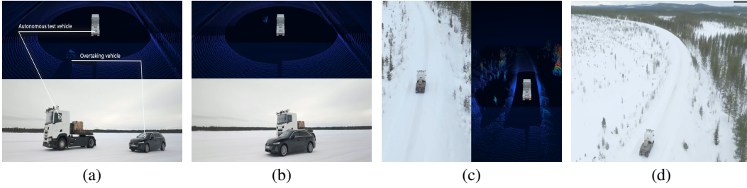
Figure 3: Real-world deployment of ICDP on a full-scale autonomous truck. (a–b) Representative multi-agent interaction trial involving an overtaking vehicle, shown from external and onboard-perception viewpoints. (c–d) Standalone driving on curved road segments under real sensing and vehicle dynamics.
