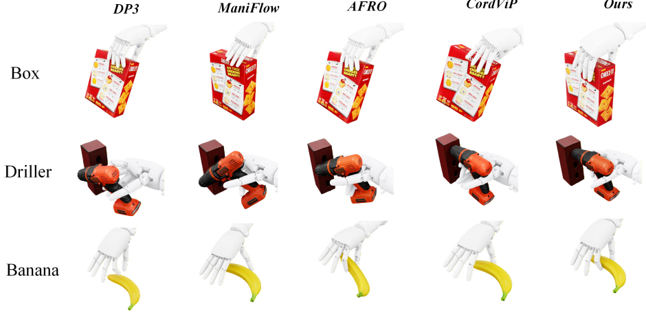
Figure 12: Visualization of hand-object interactions on the self-designed tasks, compared with typical failure cases from existing baselines.
