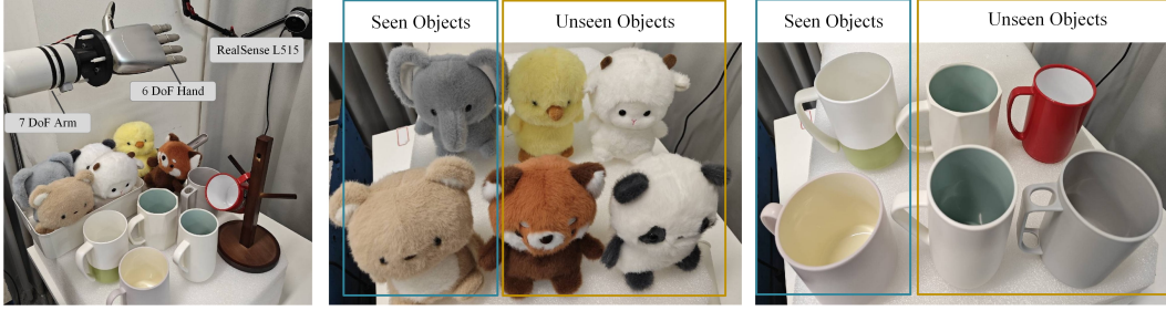
Figure 19: Real-world platform and evaluation objects. We use a RealMan RM75B arm with a 6-active-DoF dexterous hand and a fixed Intel RealSense L515 camera, and evaluate on seen and unseen objects with diverse shapes and sizes.
