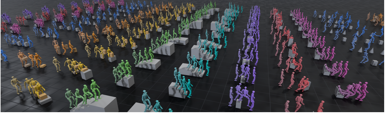
Figure 1. HIGenNTO synthesizes humanoid–scene interaction motion references through constrained optimization over a generative motion prior. Stair traversal, sitting and standing, and box pickup and placement across randomized scenes, without any motion capture of joint human–scene interaction.
