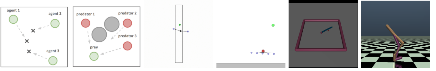
Fig. 2. Evaluation benchmarks (ordered left to right): MPE Spread and Tag, involving landmark navigation and prey interception; VMAS Buzz-wire and Balance, requiring cooperative manipulation of a shared object toward a target; and Multi-Agent Reacher and Walker2d, focusing on multi-link robotic arm control and coordinated bipedal locomotion.
