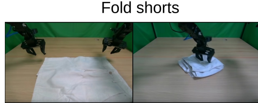
Figure 4: Robot experiments with folding shorts.
