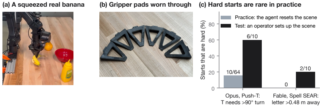
Figure 11. What hardware exposes that simulation misses. (a) A grasp that squeezes a real banana. (b) Gripper pads worn through during practice. (c) How often a task starts in a hard state: in practice, where the agent resets the scene itself, and in the test, where an operator sets it up (counts from the recorded start states).
