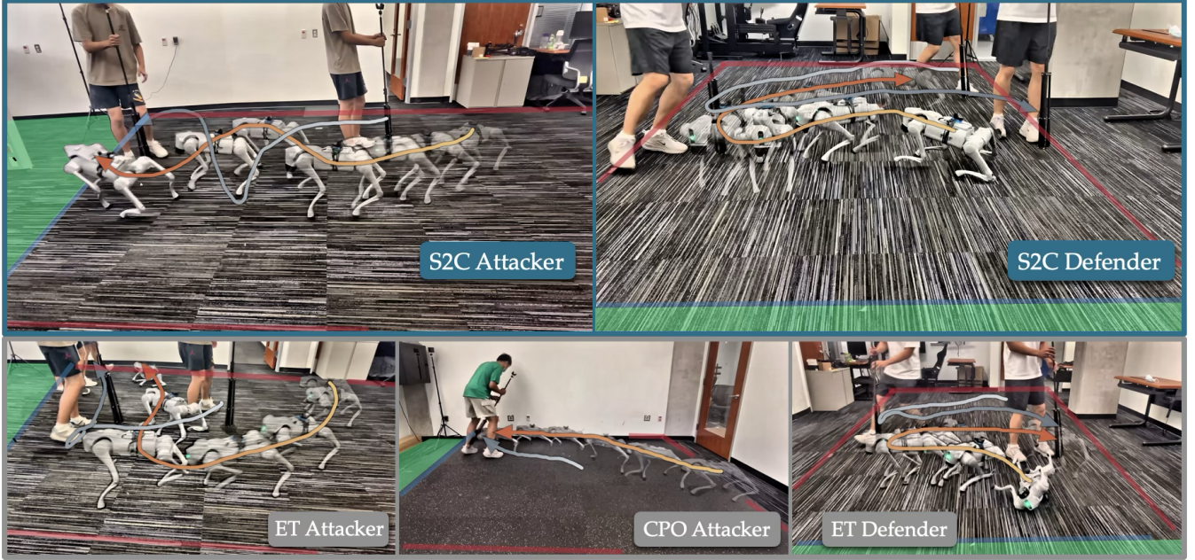
Fig. 1: Our proposed Safety to Competence (S2C) enforces robot safety without sacrificing competitive performance by training multi-agent reinforcement learning (RL) policies with a pretrained robust safety filter embedded in the environment. Here, a quadrupedal robot (orange trajectory) plays a touchdown game against a human opponent (grey trajectory), where the attacker must reach the green touchdown region before timeout; the robot loses immediately if it falls, crosses the red field boundary, or initiates a collision. Top: S2C learns effective attacking and defending tactics. As attacker, it feints past the human to score a touchdown; as defender, it tracks rapid human direction changes and holds the line. Bottom: safe RL baselines fail frequently under competitive opponent strategies: the ET attacker exits the field while turning, the CPO attacker collides with the human, and the ET defender falls while pursuing the human. Project webpage: https://alliance-ai.cs.jhu.edu/s2c/ .
