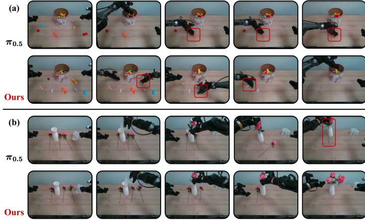
Figure 6: Qualitative comparison of real-world executions: (a) Block Collection and (b) Flower Arrangement. Each panel shows \pi_{0.5} (top) and \text{ACT}^3 (bottom), with keyframes ordered from left to right. Red boxes highlight grasping and insertion details.
