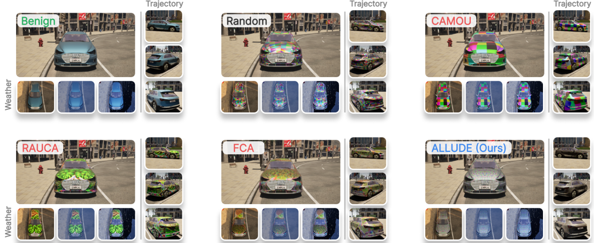
Figure 6. Comparison of adversarial textures on the Audi E-Tron under various environmental conditions. Baselines (Benign, Random), published attacks (CAMOU, RAUCA, FCA), and the ALLUDE-optimized texture is rendered across weather conditions and camera trajectories. Textures that suppress detection at clear-noon static views (top) degrade as weather (right) and viewpoint (bottom) shift.
