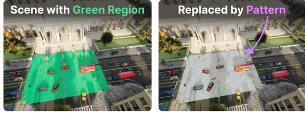
Figure 2. Existing adversarial attack evaluation “superimposes” the adversarial pattern onto the pre-determined placeholder region (here: green patch). Any overlapping objects (here: cars, shadows), are identified and replaced using their metadata. While this appears as true pattern replacement, the adversarial pattern is not rendered in the environment, thus preventing accurate evaluation.
