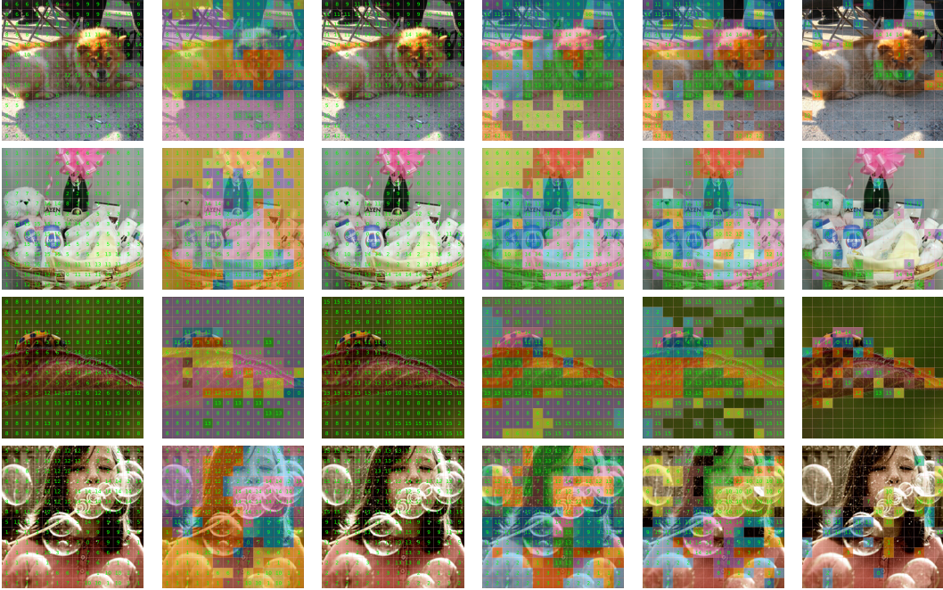
Figure 6: Patch-to-SMB assignments in our single-layer A5 classification model with a keep ratio of 0.0 and our three-layer A1A3A5 classification model with keep ratios of 0.75, 0.25, and 0.0. From left to right, the figure shows the patch-to-SMB assignments and corresponding color-coded masks at the single compression layer of the A5 model, followed by the patch-to-SMB assignments for the tokens entering the first, second, and third compression layers of the A1A3A5 model. For example, the visualization at the first layer therefore includes all input patch tokens; this layer subsequently drops 25% of them, and the retained tokens enter the second compression layer. Green numbers identify the SMB tokens assigned to reconstruct the corresponding patches, with patches assigned to the same SMB sharing the same color. Patches without a number have been dropped by preceding compression layers. The examples are randomly selected from the ImageNet validation set.
