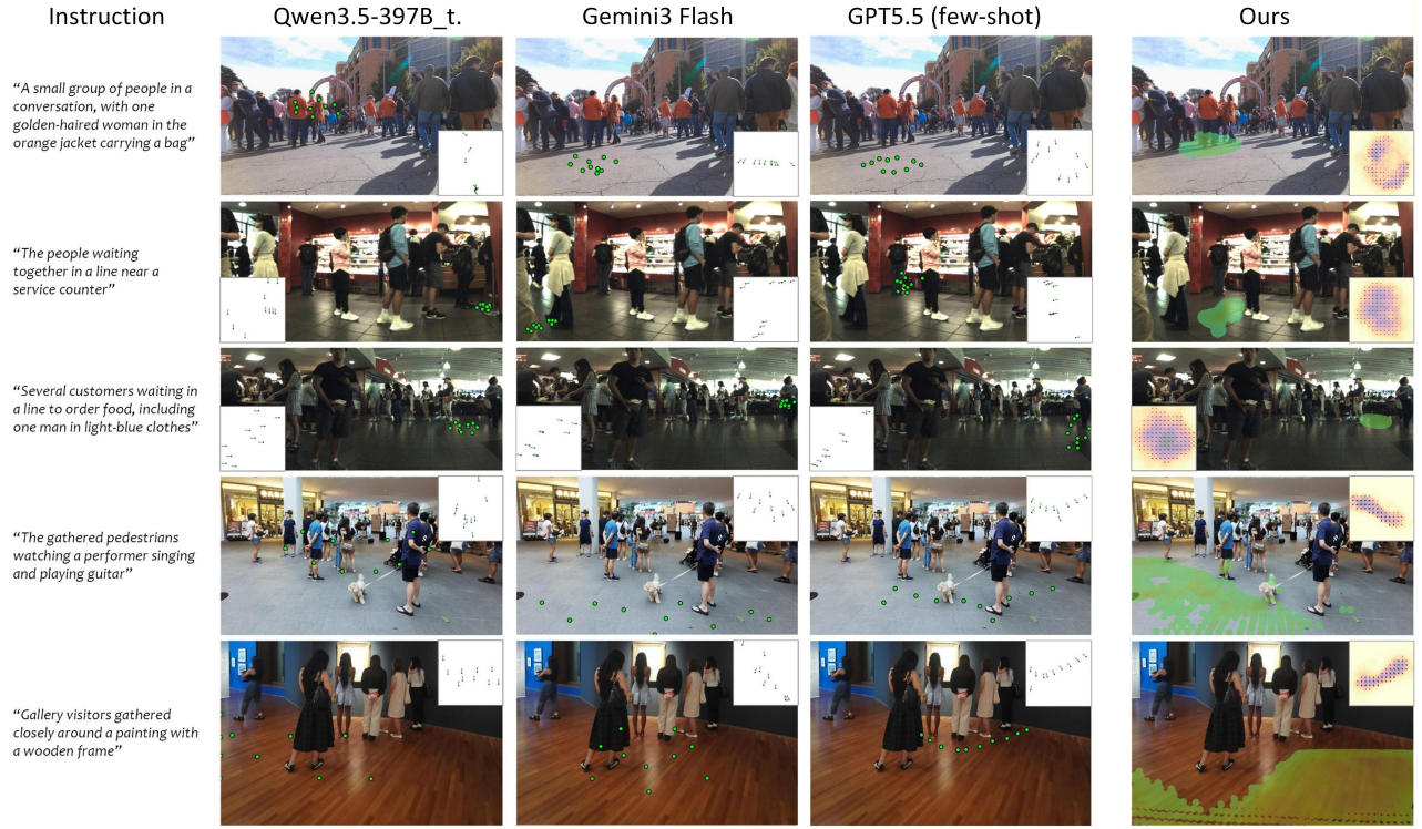
Fig. 7. Visualization of goal prediction results on offline scenarios. Orientations are displayed in small square insets for each scene. Green dots denote VLM predictions, with boundary points indicating predictions outside the image frame.
