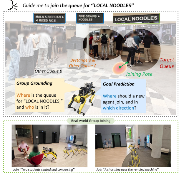
Fig. 1. Robot group joining from language instructions. Given a target group description, our method identifies the members and predicts socially compliant, geometrically valid joining poses.
