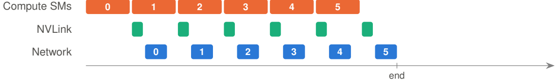
Figure 1 Three schedules for computation and communication. (a) Intra-node fusion followed by a separate inter-node collective. (b) Two streams overlap communication of completed two-tile chunks with computation of subsequent chunks; each producer-kernel boundary releases a chunk. (c) mKERNEL schedules both communication tiers within the kernel, exposing tile-level readiness signal. We note that existing compute kernels already operate on tile granularity, so GEMM efficiency is not affected. Numbers identify output tiles; widths are schematic, not measured.
