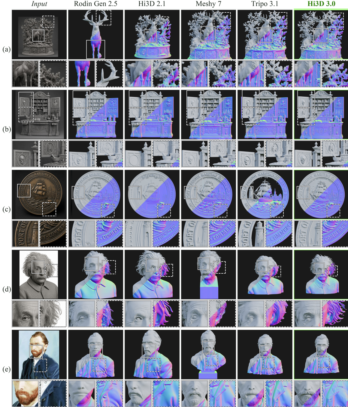
Figure 6. Five-system comparison with two close-ups per input. Each result is split diagonally, clay shading above and normal shading below. Beneath each view, the left close-up enlarges the solid white box and the right close-up the dashed white box; each box marks the same part of the object in every column, and all close-ups share one source resolution. (a) Front legs; the right-hand tree. Rodin Gen 2.5 returns the stag alone, without the niche, foliage, or base, so its right close-up shows only an antler. Hi3D 3.0, Meshy 7, and Tripo 3.1 form separate leaves and cones on the tree, which Hi3D 2.1 merges into lumpy clusters. (b) Skull and ribcage medallions on the left door. Hi3D 2.1 leaves both medallions blank; Hi3D 3.0 carves the eye sockets and teeth of the skull and separate ribs along the spine. (c) The lighthouse with the rim lettering “PORT OF”; the rim lettering “COMMERCE”. Meshy 7 and Hi3D 3.0 form both words and a windowed lighthouse. Tripo 3.1 misshapes “COMMERCE” and cuts away the inner field of the medal, leaving the lighthouse free-standing. Rodin Gen 2.5 forms “PORT OF” but garbles “COMMERCE” and forms no lighthouse. Hi3D 2.1 forms illegible glyphs and a plain tower. (d) Eye and forehead; side hair. Hi3D 3.0 forms separate tapered strands and a carved iris, where the other systems form clumps, ribbons, or smooth sheets; Meshy 7 also truncates the bust at the neck. (e) Beard; collar and buttons. Hi3D 3.0 and Meshy 7 form beard strands and curls, and Rodin Gen 2.5 forms no beard; all five systems reproduce the collar and buttons. Meshy 7 adds a plinth that is not in the input to both busts.
