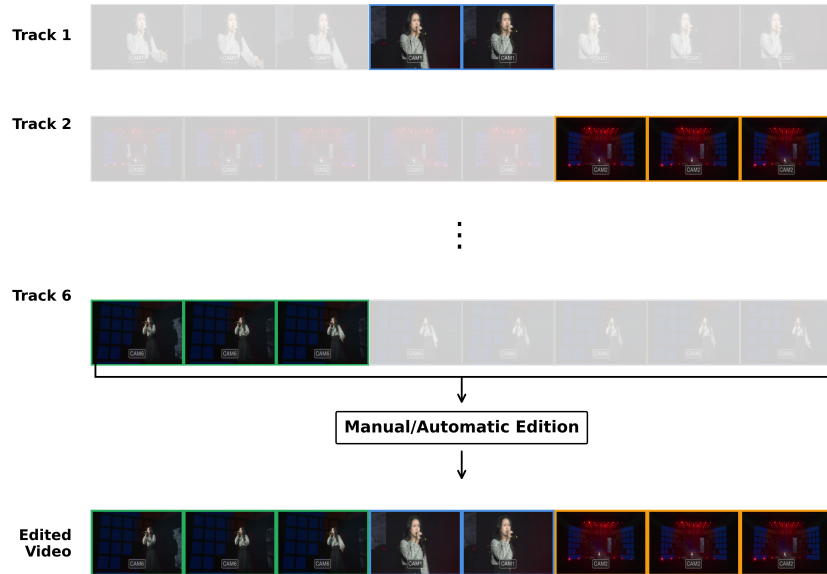
Fig.1: Overview of the multi-camera editing process using an example from the TVMCE dataset [13]. A professional editor (or an automated system) selects the most appropriate viewpoint from multiple concurrent camera tracks (shown here as Tracks 1, 2, ..., 6) to construct a final edited sequence that maintains narrative and visual continuity.
