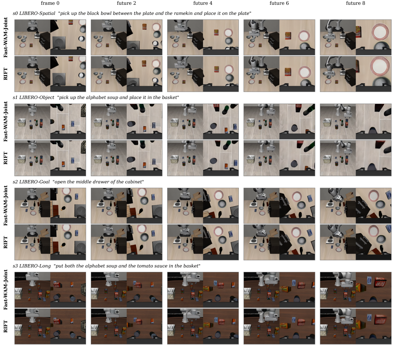
Figure 8: Imagined future: Fast-WAM-Joint iterative diffusion versus RIFT one pass. Per state, the top strip is Fast-WAM-Joint’s future decoded from its full iterative diffusion rollout; the bottom strip is decoded from RIFT’s anticipation tokens after one backbone pass. The first column is the shared current observation at frame 0; the remaining columns show decoded frames 2, 4, 6, and 8. Visual similarity is illustrative; policy behavior is evaluated separately.
