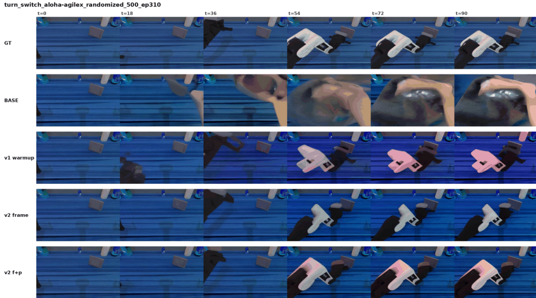
Figure 20: Training evolution on turn_switch (ep310). EVAC-v1 produces a reddish robot arm, a bluish background, and implausible floating-arm geometry. EVAC-v2 Frame substantially reduces the color bias, but the arm shape remains distorted. EVAC-v2 Fr.+Patch further improves the local arm geometry and produces an embodiment substantially closer to the ground truth.
