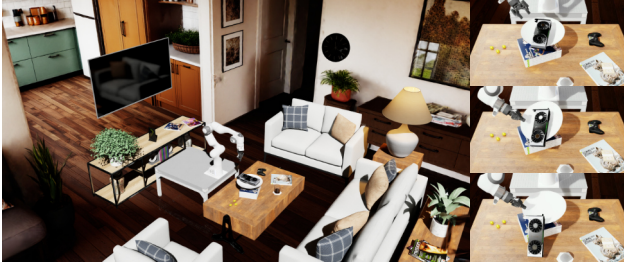
Fig. 9: (Left) We show one of our Gaussian Splat + Mesh scenes in RoboLab. This scene has a Gaussian splat background with a collision mesh for the splat estimated with 3DGRUT [22, 30], and a mesh foreground. All objects in the scene have spatially varying density, and thus mass is estimated with VoMP [6]. (Right) We show a VLA running a task in this scene.
