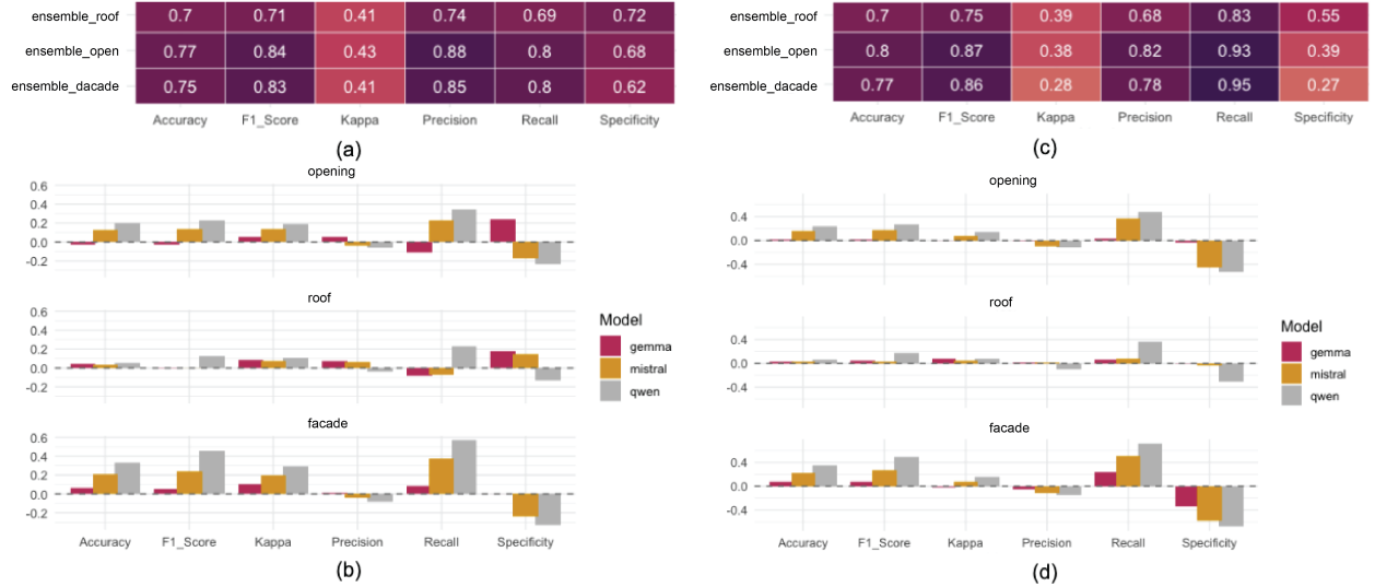
Figure 6: Comparison between ensemble and base models based on the test set: the performance of the ensemble learner and base models with threshold selected for maximizing kappa (a) and for maximizing F1-score (c); (b) the delta between the performance of the ensemble learner and base models with threshold selected for maximizing kappa (b) and for maximizing F1-score (d)
