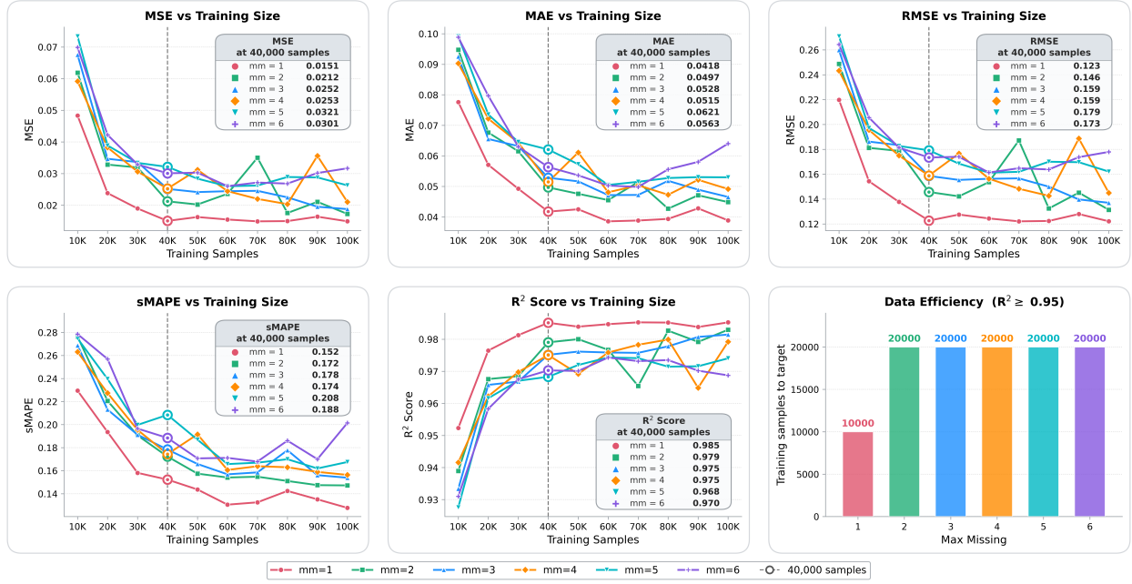
Figure 7: Learning curves for random sampling baseline across all MM levels. Performance metrics (MSE, MAE, RMSE, sMAPE, R^2 ) are shown as a function of training size (10,000–100,000). Insets report each metric at the 40,000-sample checkpoint (dashed line). The bottom-right panel shows the number of training samples required to reach R^2 \geq 0.95 at each MM level. A performance plateau is reached around 40,000 samples.
