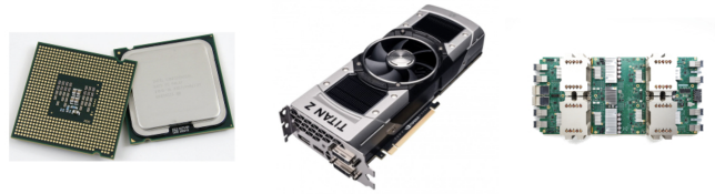
Fig. 7.9 CPU, GPU, and TPU
