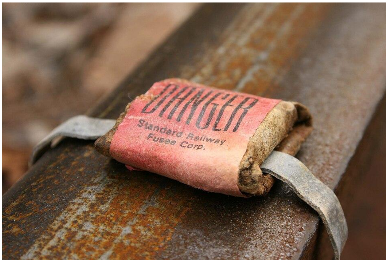
Figure 1. A railroad torpedo with its lead straps, the American counterpart of the British detonator. The straps hold the charge to the rail head; a passing wheel fires it, so the warning works when signals and sightlines fail. Photograph by Ralph Mayer, licensed under CC BY 2.0.
