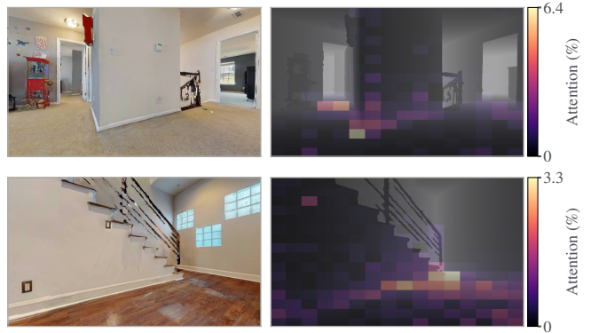
Fig. 4. Summarizer attention pattern on two sampled frames from evaluation scenes. Left: RGB images, for reference only. Right: attention of the summarizer’s learned query token over patch tokens, averaged over attention heads and overlaid on the depth image.
