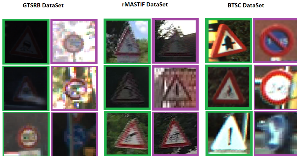
Figure 15: Prediction of RIECNN model on the three datasets, focusing on challenging test set images. Green background indicates correct prediction, purple background indicates miss-classification
