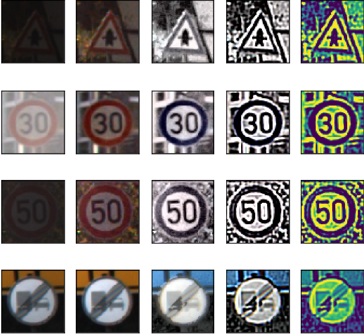
Figure 1: Sample of GTSRB traffic signs after pre-processing, left images are original unprocessed ones and the next images to the right display the result after each stage of pre-processing in order: 1) Image contrast enhancement, 2) Retinex algorithm, 3) Histogram equalization, and 4) Edge enhancement with gray-scale conversion
