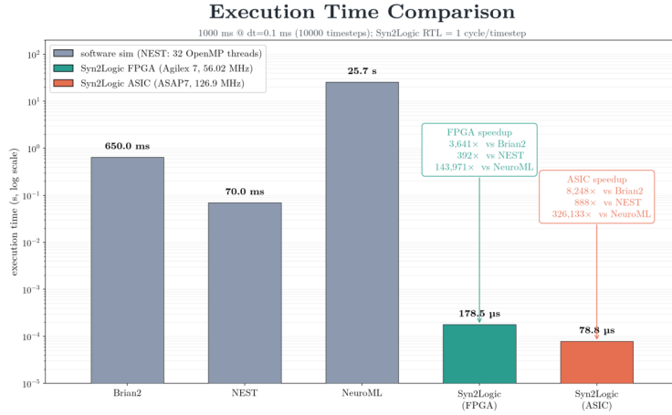
Fig. 7: Performance comparison between simulation and Syn2Logic FPGA and ASIC auto-generated C. elegans accelerators.
