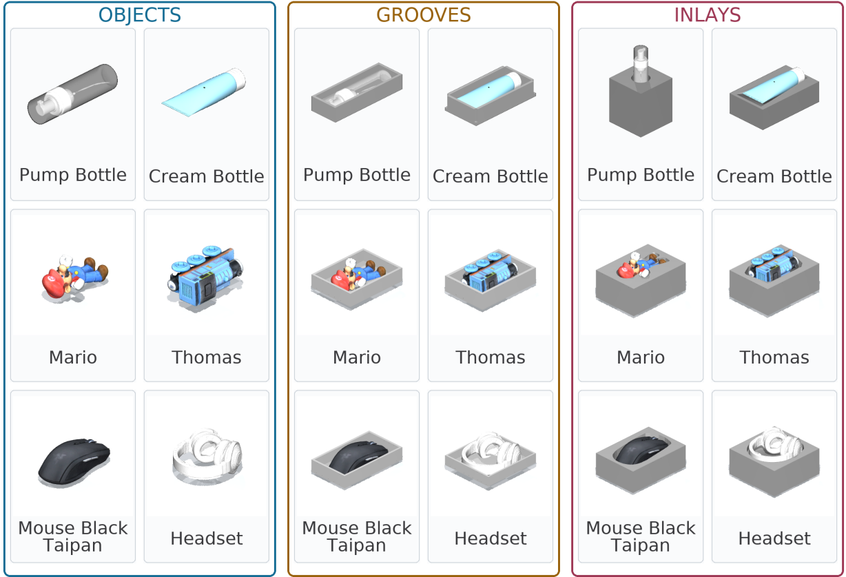
Figure 6: Representative LIBERO-Industry workpiece and fixture assets. From left to right, the panels show six evaluation workpieces and their object-specific Level 2 grooves and Level 3 form-fitting inlays, spanning personal care, model figurines and vehicles, and consumer-electronics domains.
