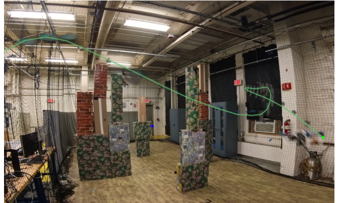
Fig. 6: Real world trajectory flown by the baseline policy. The drone drifts toward the net to the side of the course, crashes into it, and never reaches the goal.
