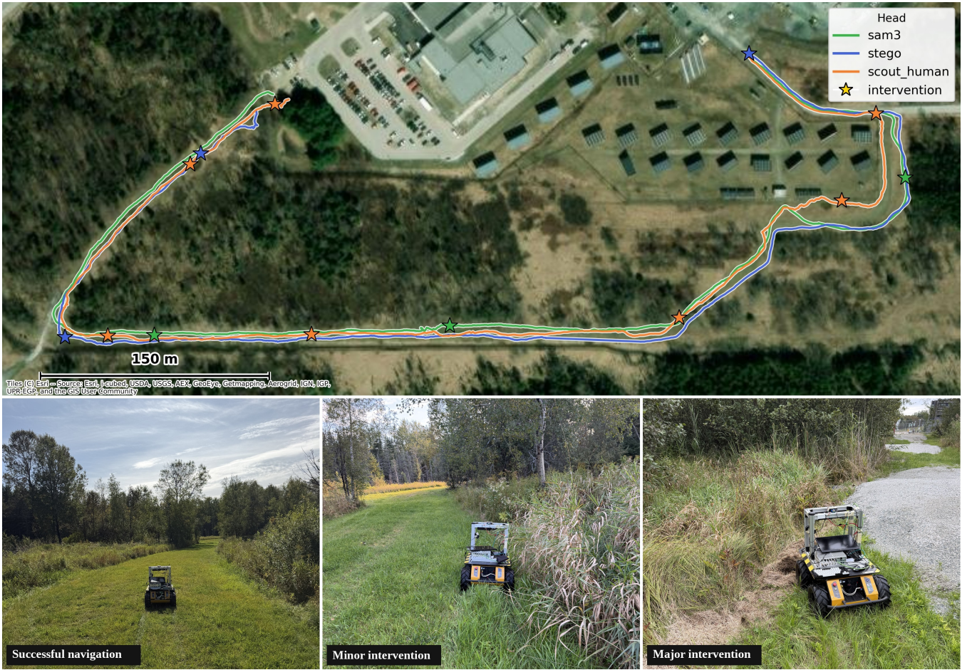
Fig. 4. GPS trajectories for stego, sam3 and HLTM heads on the identical route and planner, overlaid on a shared basemap. Clustered operator-intervention episodes are marked per head. Added below are example interventions: successful navigation, a minor intervention near the trail edge, and a major intervention into high grass.
