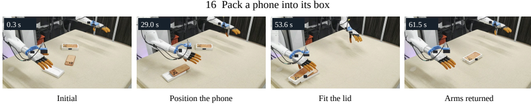
Figure 10: Additional recorded task sequence (III). Task 16 packs a phone into its box and fits the lid. The four original-video frames show the initial configuration, phone positioning, lid placement, and the final configuration with both arms returned. Torso and incidental packaging and equipment text are masked; timestamps refer to the source video.
