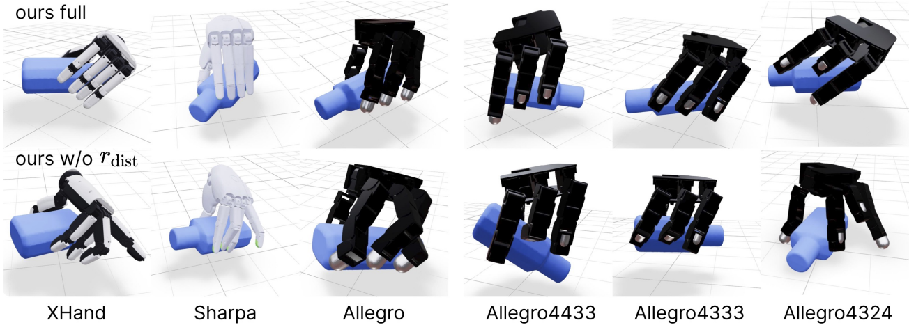
Figure 6: Qualitative grasps on training and unseen embodiments. We compare the full GOTT (top) with the variant without r_{\text{dist}} (bottom) on three training hands and three unseen Allegro variants.
