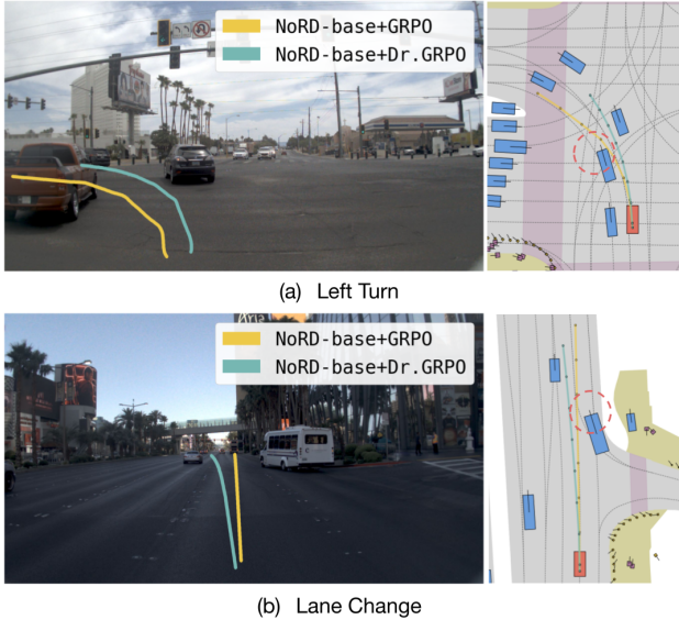
Figure 4. Qualitative comparison of RL fine-tuning (RLFT) on the weak SFT model using GRPO and Dr. GRPO. With Dr. GRPO, NORD successfully learns complex maneuvers such as sharp turns and lane changes without collisions, whereas GRPO fails to optimize the weak SFT model (NORD-BASE) and collides (in red).
