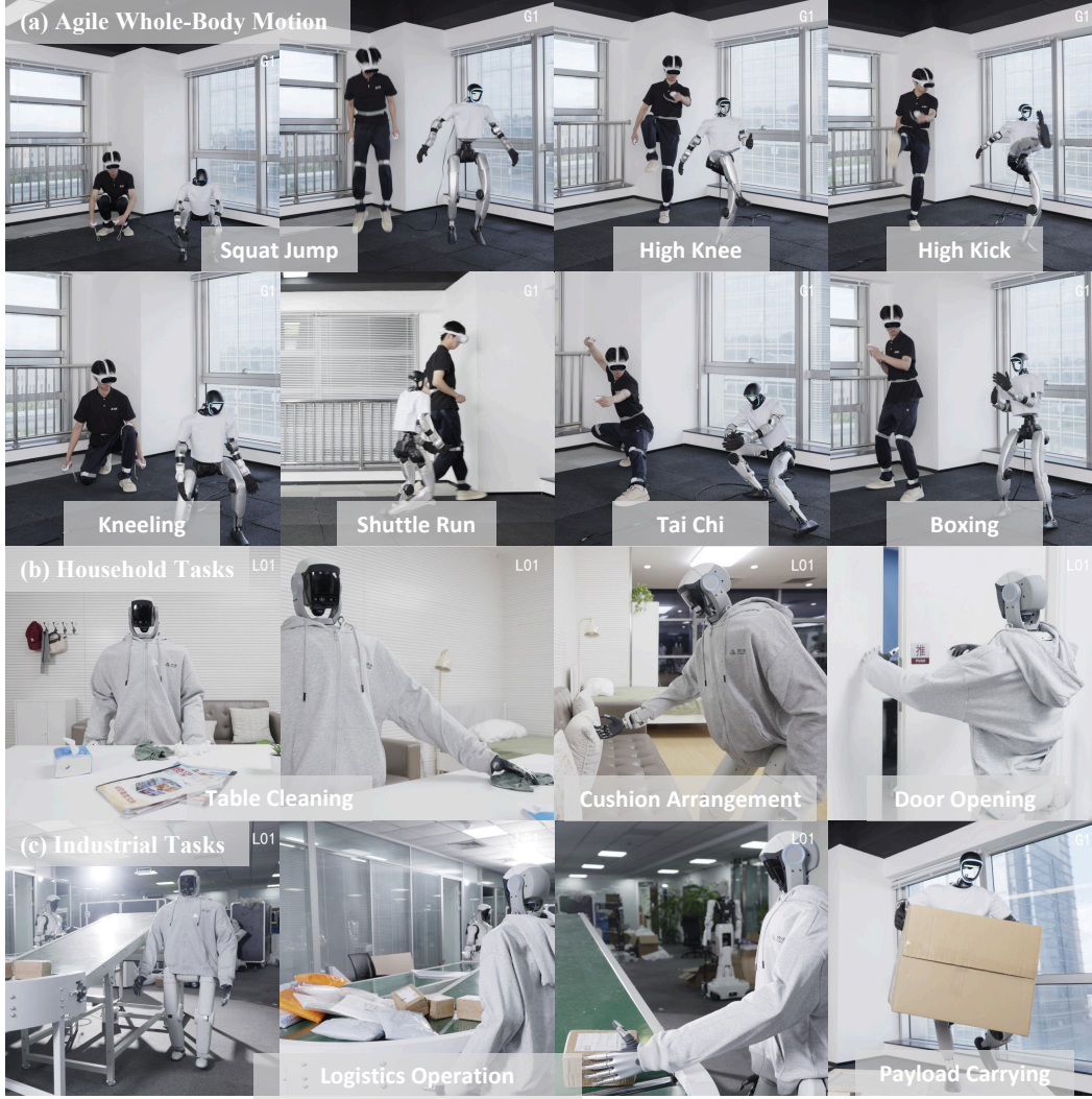
Figure 8. Whole-body motion capability. Agile motion, household tasks and industrial tasks, all produced by one tracking policy under live whole-body command. Frames are badged with the robot they were recorded on: the controller runs on a Unitree G1 and, after the fine-tuning of Section 3.5 , on a Maker L01.
