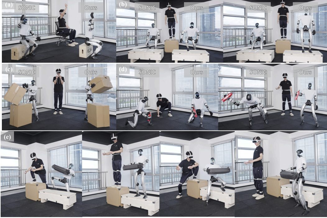
Figure 5. Environment interaction on hardware. Matched hardware comparisons in (a)–(d), with SONIC [23] on the left and GigaBrain-WBC-0.5 on the right, driven simultaneously by the same operator command. (a) Ours loads the box as a seat while SONIC remains in a half-squat. (b) Ours steps onto the platform and stabilizes; SONIC fails to climb it. (c) Ours lifts and holds the box while SONIC loses a stable grasp. (d) Ours completes a kneel-to-stand transition to lift a 2 kg fire extinguisher while SONIC falls during the rise. (e) Ours carries a large case while walking forward onto the platform and down to the floor.
