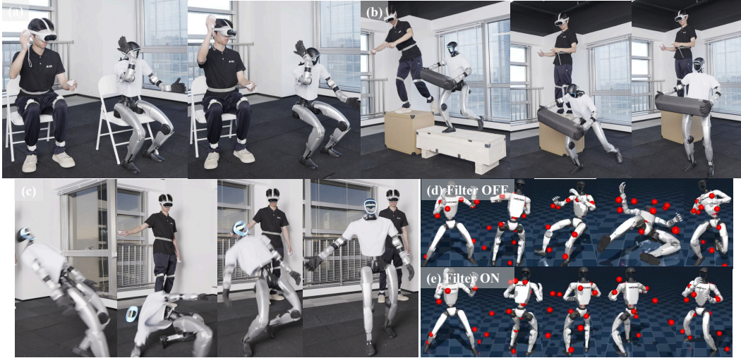
Figure 7. Robustness to unsafe commands and to physical disturbances. (a, b) Removing the chair or platform invalidates the original command, yet the policy settles into a stable best-effort behavior instead of an emergency stop, in which case the carried object would be dropped. (c) The same tracking policy recovers from a kick-induced fall without a separate recovery controller. (d, e) Under the same self-interfering and challenging spinning-kick reference in simulation, disabling the safety filter causes the robot to attempt the kick and fall (though subsequently recover); enabling it preserves the commanded turn, suppresses the difficult kick and keeps the robot upright.
