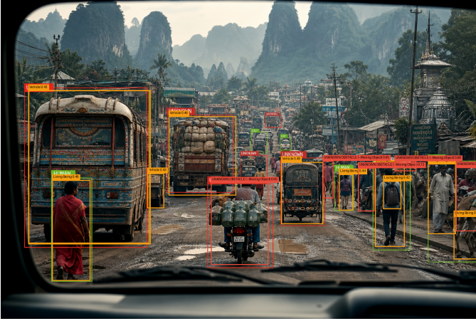
Fig. 1. The hierarchical layer on a road scene. Each region carries the most specific safe taxonomy level the evidence supports, or an explicit UNKNOWN OBSTACLE; it never attaches a confident wrong specific label.
