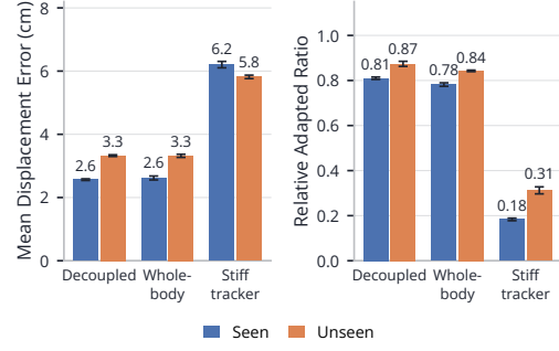
Fig. 3: Evaluation results on compliance interaction. Under force, both compliant policies move the wrist most of the distance encoded in the adapted reference, while the stiff tracker moves it far less. Error bars show the standard deviation over evaluation seeds.
