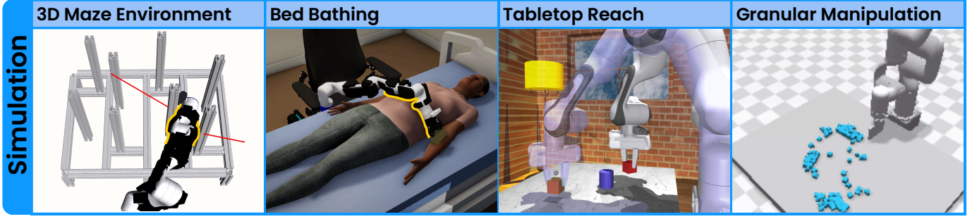
Fig. 3: Simulation task suite. We evaluate TACTIC across four simulation environments: the 3D Maze Environment tests whole-arm navigation through a maze, analogous to navigation in a cluttered environment; Bed Bathing tests task execution of wiping a person in bed with incidental whole-arm contact; Tabletop Reach tests obstacle-aware reaching across a table; and Granular Manipulation tests contact-driven rearrangement of small particles. Whole-arm contact is highlighted in yellow.
