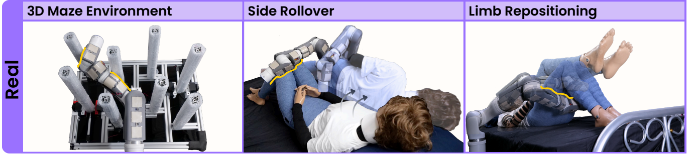
Fig. 4: Real-world task suite. We evaluate across three real-world environments. The 3D Maze Environment tests whole-arm navigation through static and dynamic obstacles, Side Rollover tests contact-rich manipulation to rotate a person while regulating interaction forces, and Limb Repositioning tests multi-contact support during lifting and repositioning of the legs to a target configuration. Whole-arm contact is highlighted in yellow.
