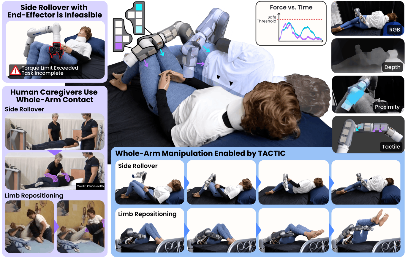
Fig. 1: TACTIC enables robots to perform contact-rich manipulation by utilizing the entire arm surface. While end-effector-centric control is often infeasible and unsafe under high payloads, TACTIC fuses multimodal observations such as RGB-D, proximity masks, and distributed tactile sensing into a contact-centric representation to enable whole-arm manipulation. We demonstrate its effectiveness on manipulation tasks, including side rollover and limb repositioning on a life-size manikin.
