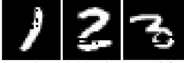
Fig. 2: Three adversarially perturbed digits (up to 100 pixels flipped). The models before adding constraints predict 2, 3, and 4 respectively, but the original labels are different. CG4AI adds constraints to enforce correct classification of these perturbed inputs.
