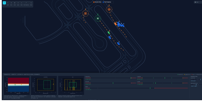
Fig. 4: The PUFFERDRIVE-EDITOR user interface. The upper panel displays the map canvas and vehicle trajectory paths (e.g., analyzing the reactive policy in orange). The lower panel contains the real-time kinematics dashboard, showing the active passenger-comfort limits (green/amber boxes) for acceleration and jerk, the vehicle’s actual realized state trajectory (highlighted dots and trail), and target action re-discretization intervals.
