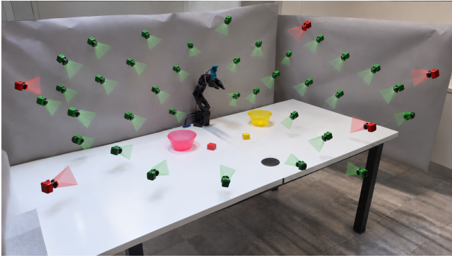
Fig. 2: Multi-view reconstruction and novel-view sampling. Red cameras are used for reconstruction; green cameras denote sampled novel views.
