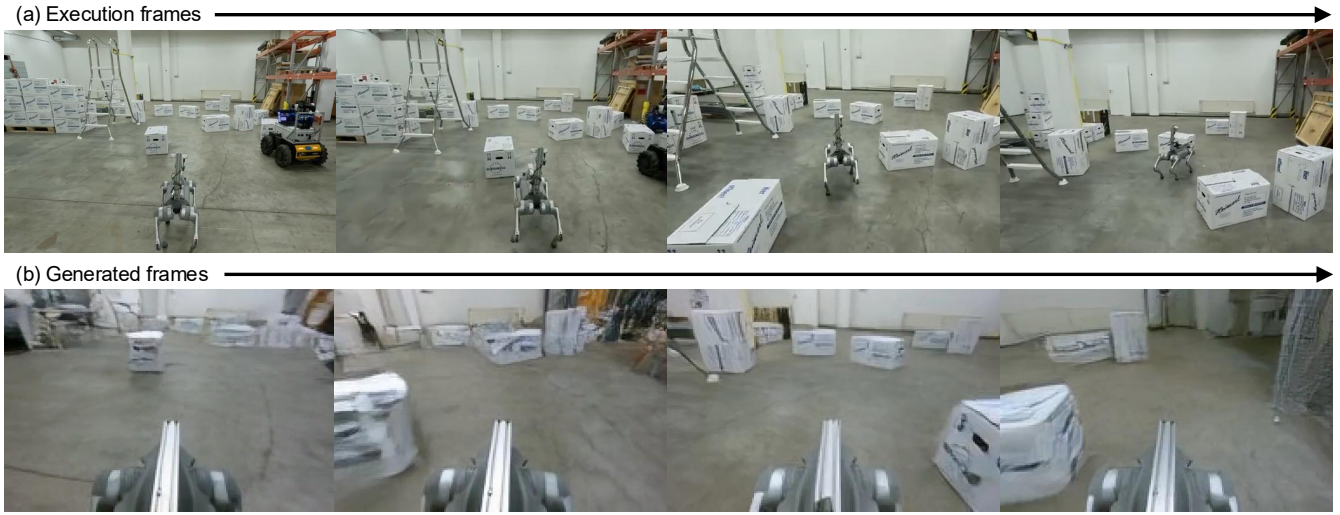
Fig. 10: Cross-embodiment deployment of CueNav on the Unitree Go2. (a) Execution frames during zero-shot navigation in a cluttered environment. (b) Corresponding generated future observations, demonstrating reuse of the shared video planner on a different robot embodiment.
