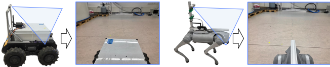
Fig. 3: Embodiment-aware observation with part of the robot body visible as a visual cue.
