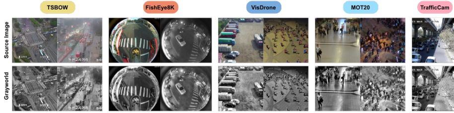
Fig. 2: Visual comparisons of raw pre-training dataset images alongside their corresponding Grayworld-augmented variants. By neutralizing sensor-specific white-balance variances and volatile RGB distributions, the Grayworld transformation effectively bridges color and style discrepancies across disparate source domains.
