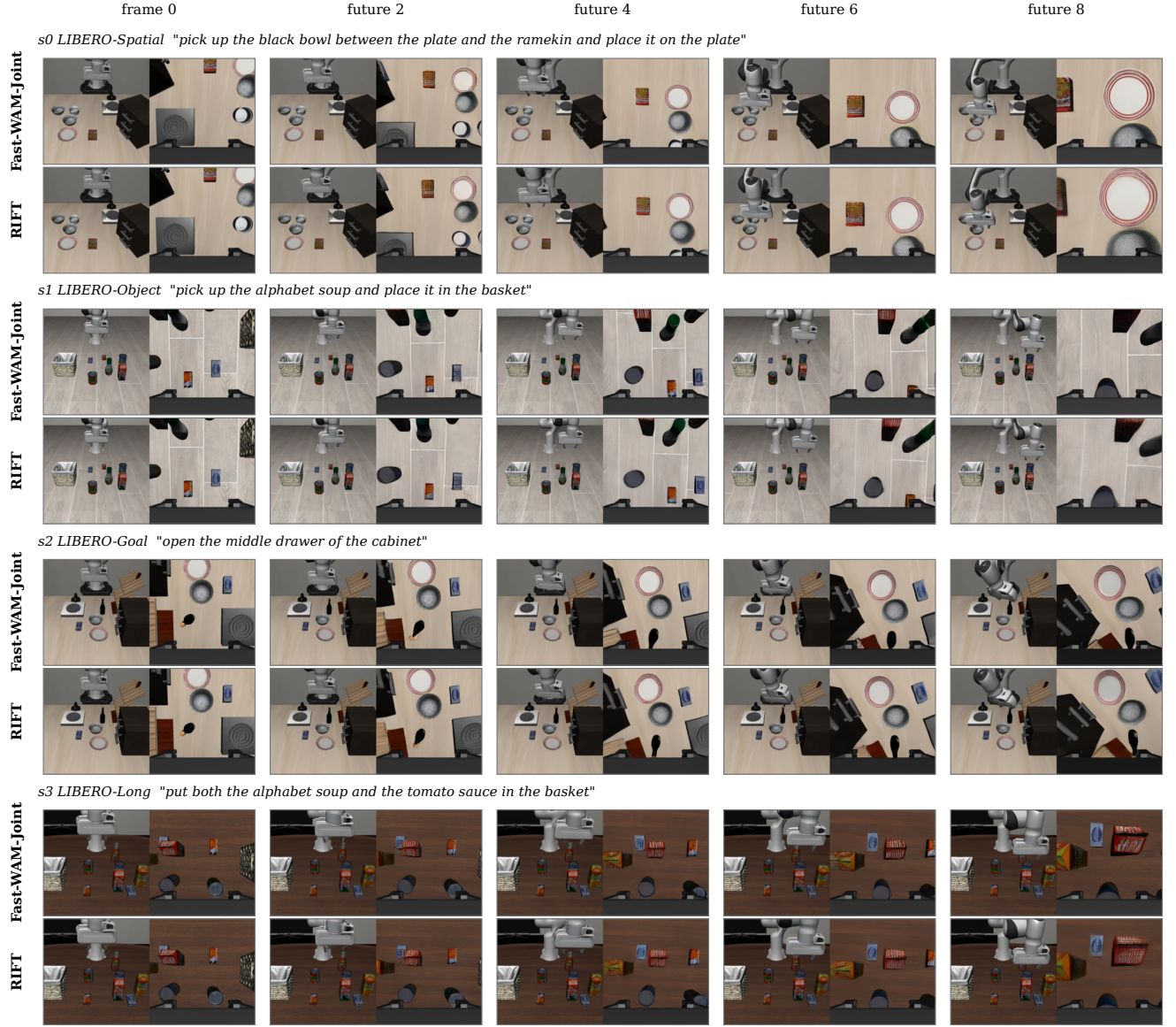
Figure 7: Imagined future: Fast-WAM-Joint iterative diffusion versus RIFT one pass. Per state, the top strip is Fast-WAM-Joint’s future decoded from its full iterative diffusion rollout; the bottom strip is decoded from RIFT’s anticipation tokens after one backbone pass. The first column is the shared current observation at frame 0; the remaining columns show decoded frames 2, 4, 6, and 8. Visual similarity is illustrative; policy behavior is evaluated separately.
