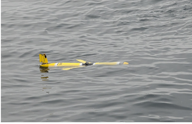
FIGURE 1: Slocum glider in operation during the eSWEETS 3 field deployment. The proposed Glider Autonomy Long-term Planning Engine system was used to pilot gliders autonomously in two long-term deployments totalling approximately 3 months and 1000 km.
