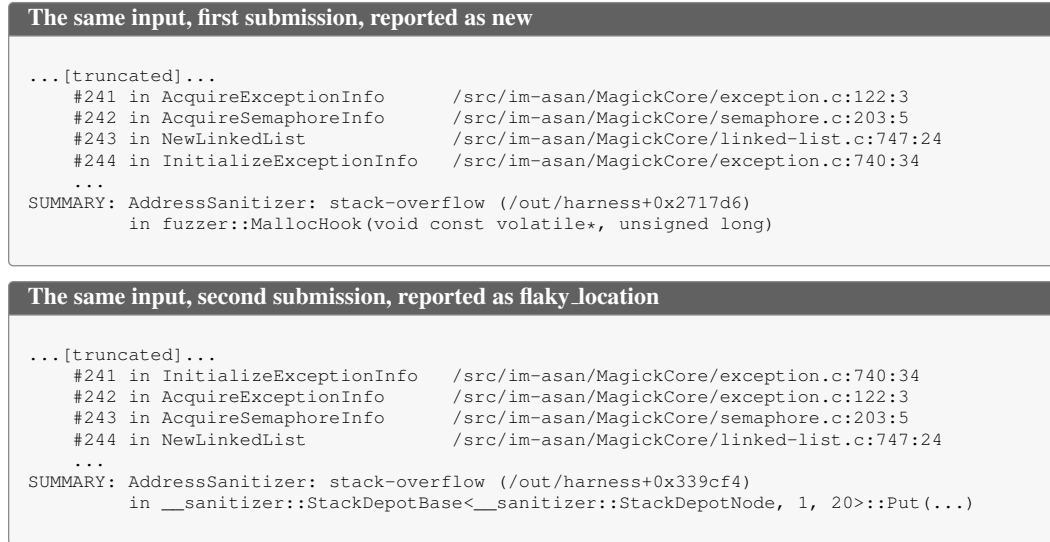
Figure 13: Two submissions of the same stack-exhaustion input in one challenge run. The first produced one signature in all three verification rounds and was accepted as new. The second produced two signatures across its three rounds and was returned as flaky_location .
