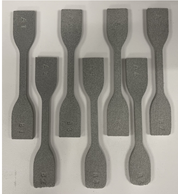
Figure 15: Initial set of tensile samples (Batch S) printed with Nylon 12 Blend (25% PA12 GF and 75% PA12 White by volume) exhibits a relatively lighter color than Material 1 or Material 2.
