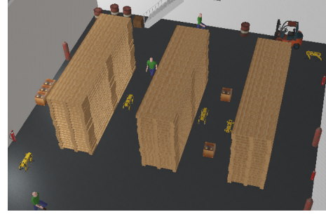
Fig. 3. Webots warehouse simulation environment with five Spot robots and a mixture of objects. Occlusions from shelves and dynamic human agents create partial observability and asymmetric sensing among robots.
