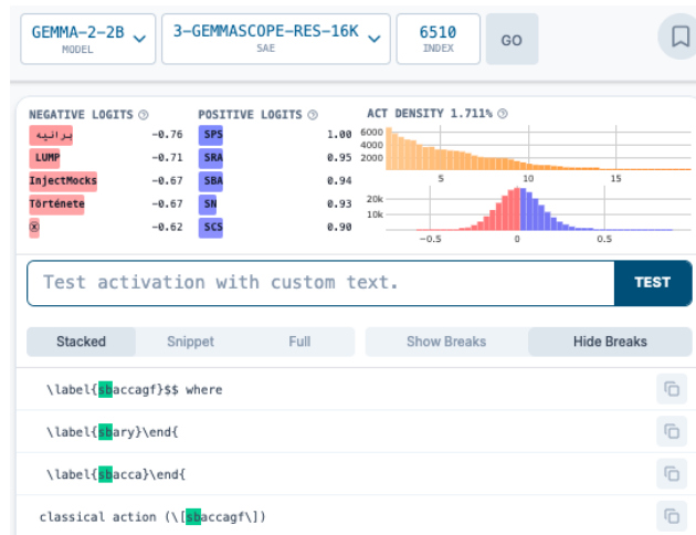
Figure 25: Neuronpedia dashboard for Gemma Scope layer 3, latent 6510. This latent should be the main “starts with S” latent.
