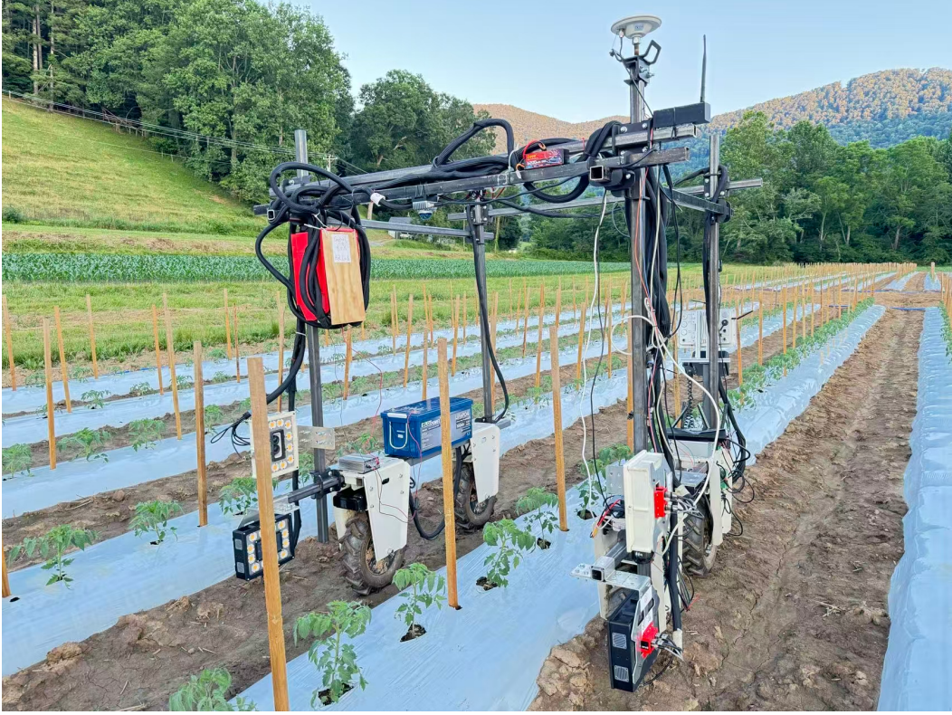
Figure 2: The customized robotic platform used for collecting disease images in a tomato field.
