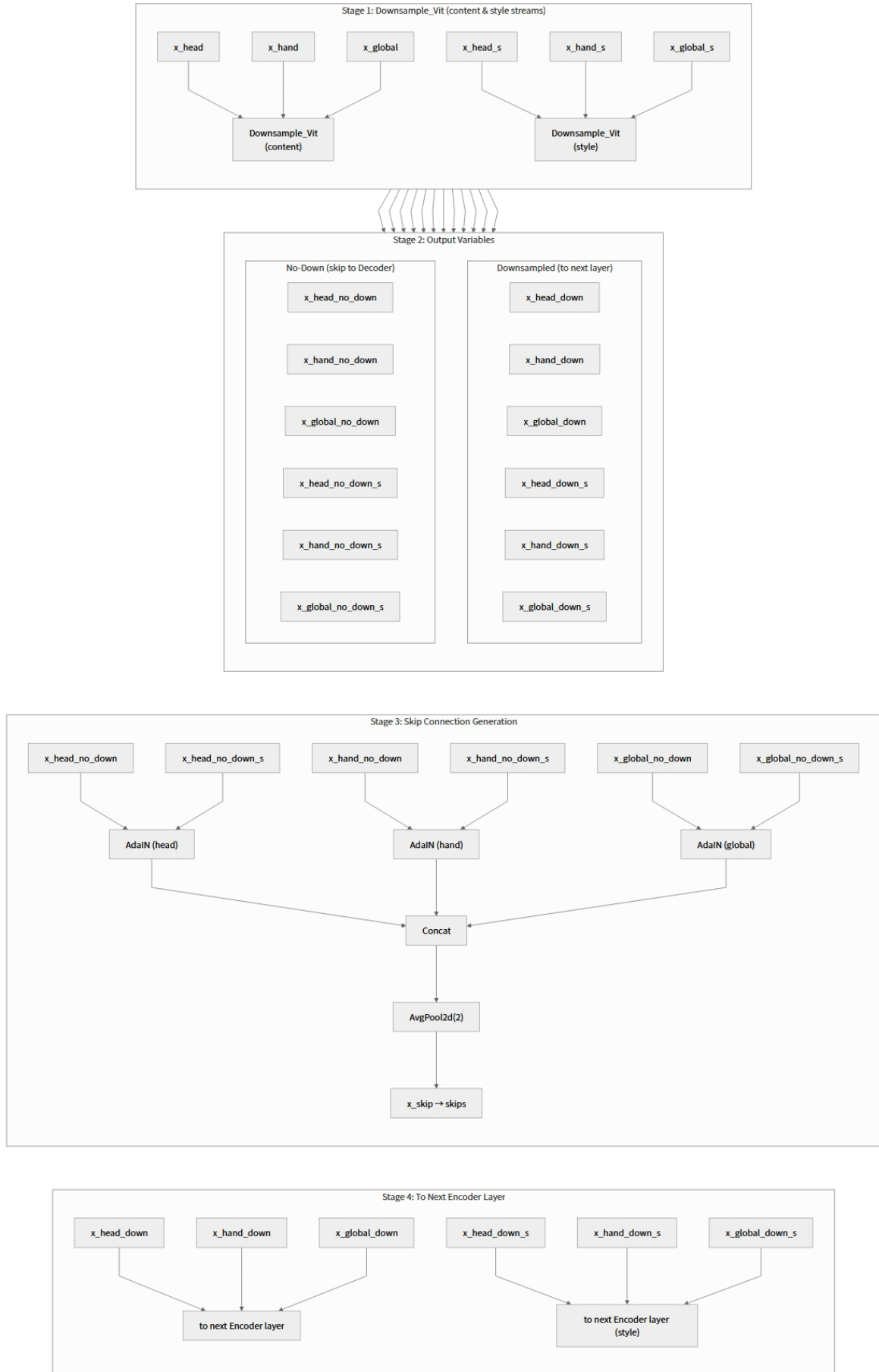
Figure 1: Encoder architecture with three parallel branches (head, hand, global). Each branch processes identical input through independent dual-pathway Downsample_Vit blocks. AdaIN fuses content and style streams at each level to produce skip connections.
