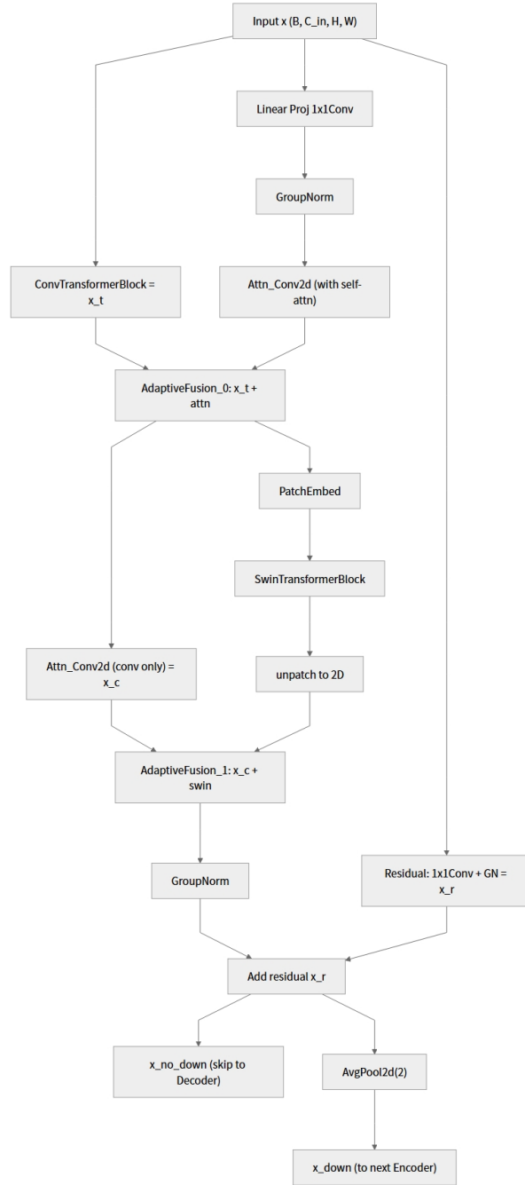
Figure 3: Downsample_Vit: dual-pathway convolutional-transformer block. Each encoder layer employs a two-stage design: Stage 1 fuses a ConvTransformer stream with a convolutional-attention stream, and Stage 2 fuses a pure-convolution stream with a Swin Transformer stream, each via learnable AdaptiveFeatureFusion, with a residual connection and 2\times downsampling.
