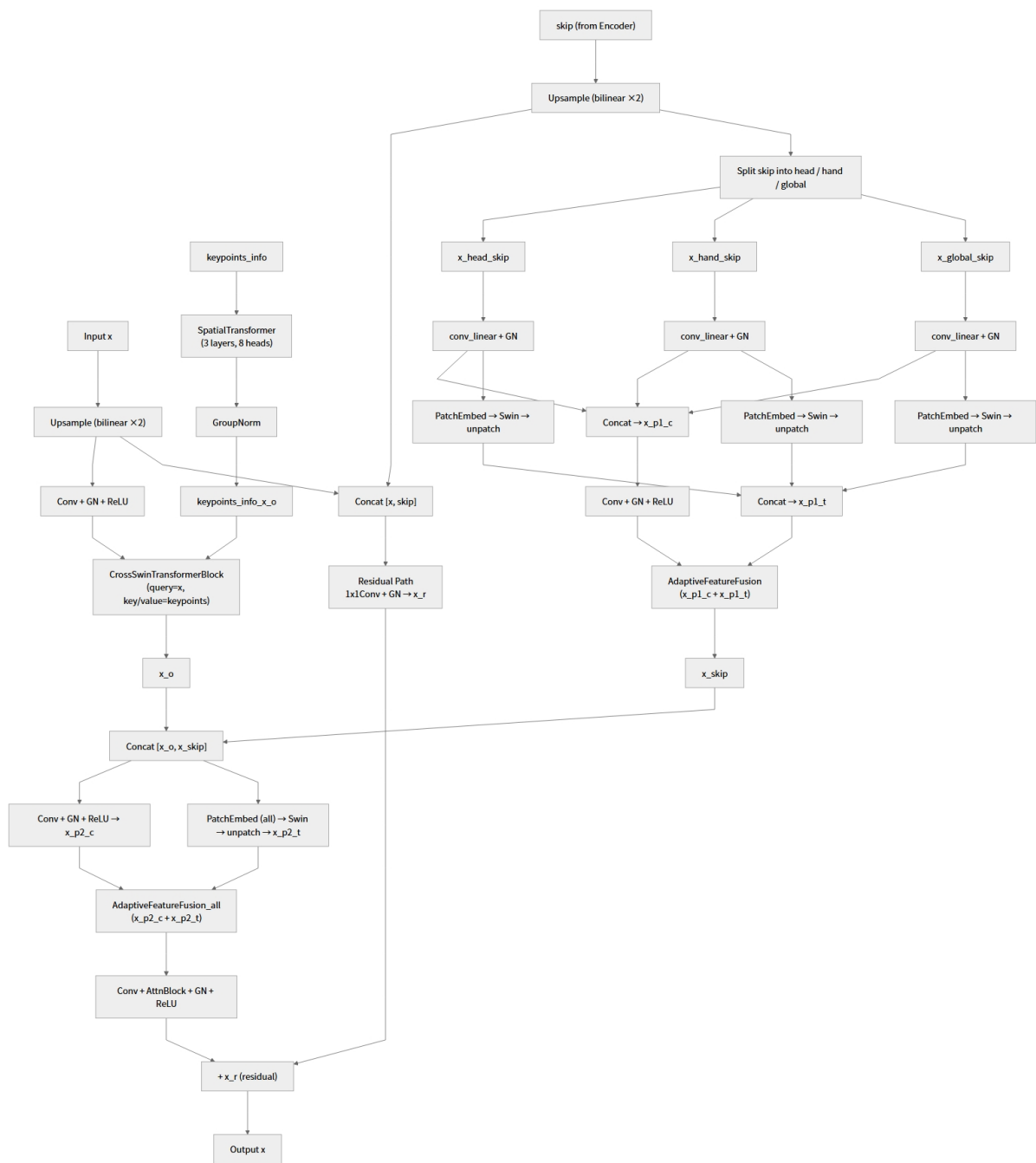
Figure 4: Upsample_Vit: dual-pathway decoder block with skip injection.
