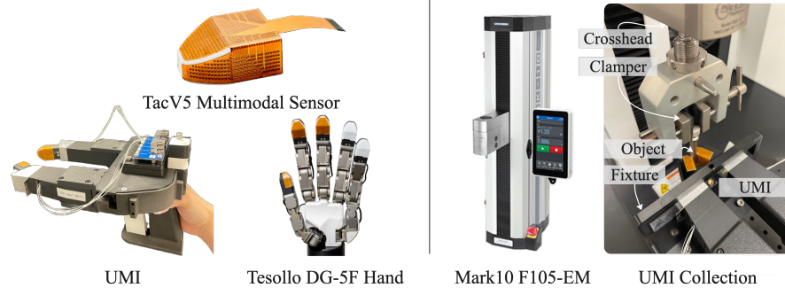
Figure 2: Left: TacV5 multimodal sensors on UMI grippers and the Tesollo DG-5F dexterous hand at the thumb, index, and middle fingers. Right: Data collection platform. The UMI is mounted on a separate table to physically isolate vibrations from the Mark10 and constrained by a fixture to suppress slip-induced shaking. Objects are secured with an adjustable clamp, while controlled slip is generated through programmable vertical crosshead motion. The operator controls only gripper opening and closing. No external camera is required.
